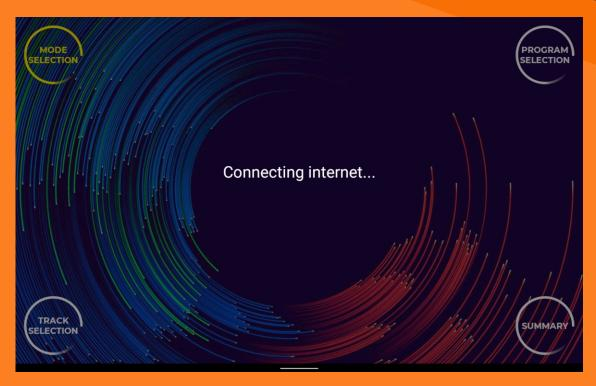
Treadmill needs to be connected to WiFi and speed internet at least 2MB. Offline mode is working 90 minutes and machine is locked until WiFi connected.
