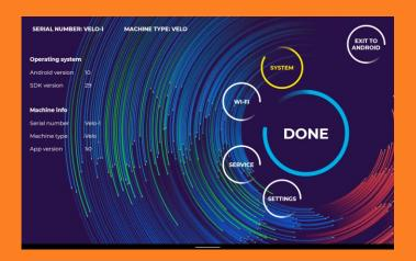
In order to get to the service functions of the device, you need to press [MENU] in the home screen. Some versions have a HIDDEN Button which you need out your finger in right bottom corner of display and hold 3-5 seconds for open HIDDEN menu.
